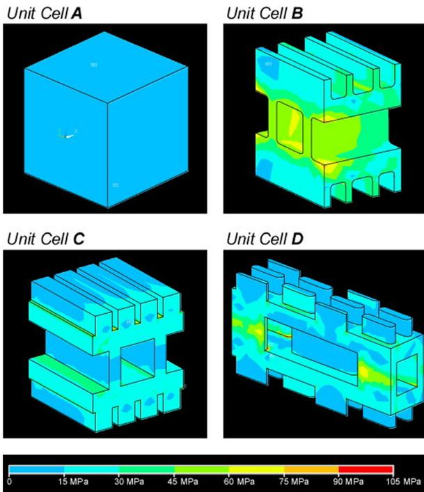
**Fig. 9** Local peak stresses on unit cells in the PCHX during a simulated thermal transient involving loss of forced liquid cooling
