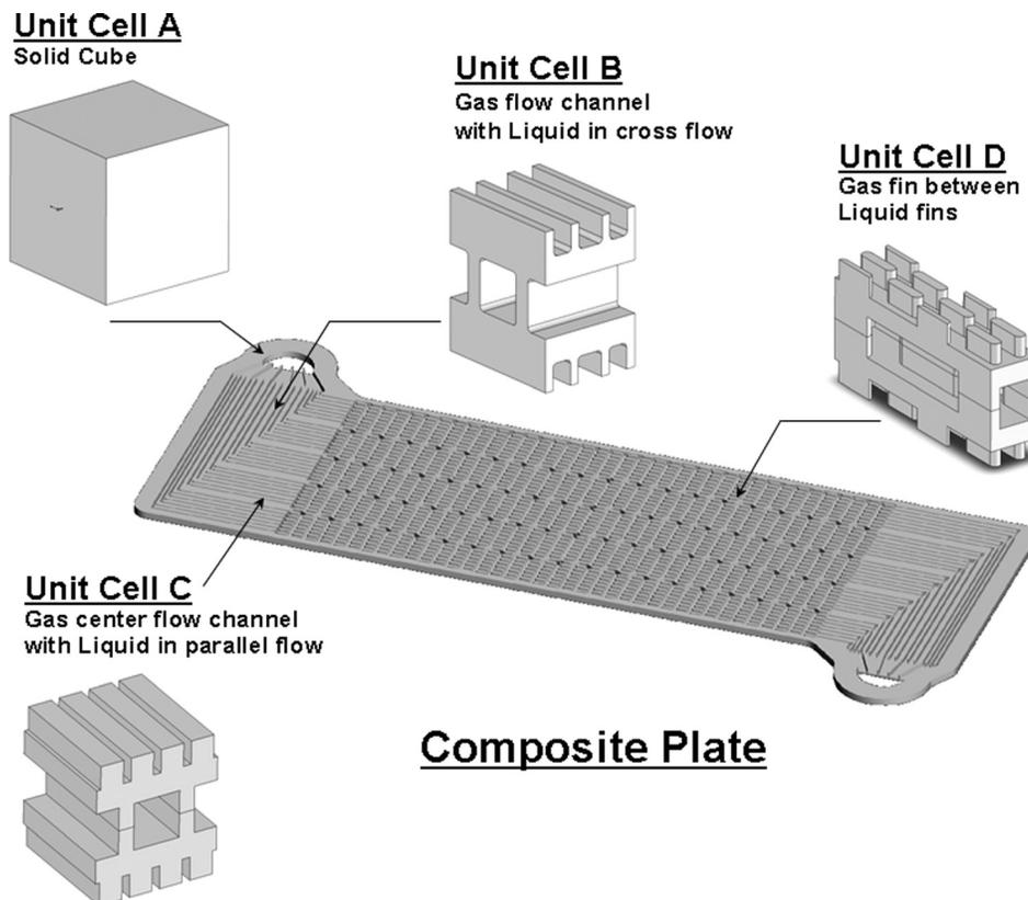
Fig. 7 The four unit cells characterizing the complex geometry of this composite plate
