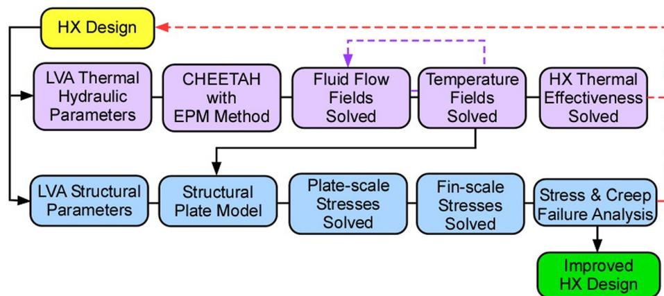
Fig. 1 Heat exchanger design optimization process enabled using CHEETAH and the EPM method
