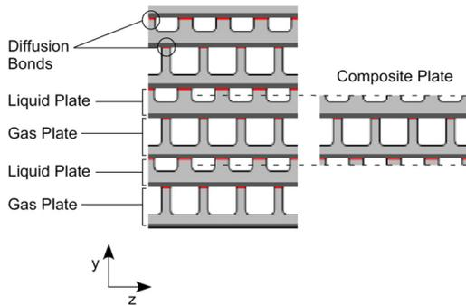
**Fig. 2** Cut-away view through the OSF section showing alternating liquid and gas flow channels. Dark bands at the top of each fin indicate the location of diffusion-bonded joints between the plates.
