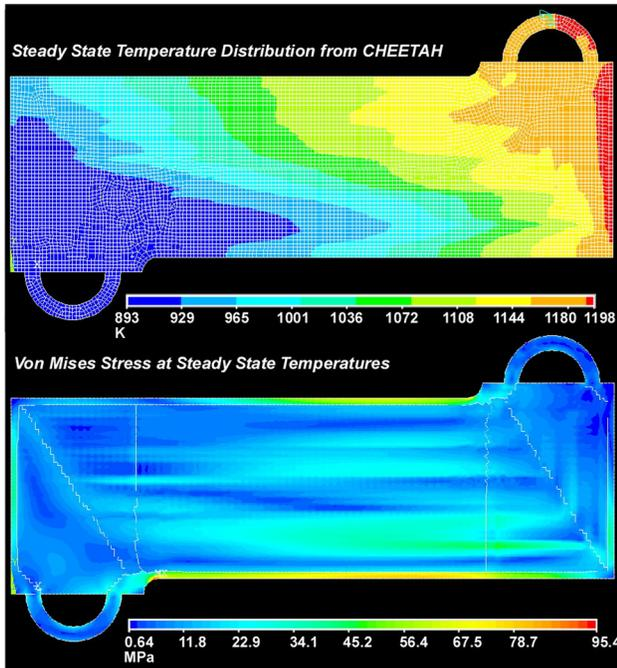
Fig. 4 The steady state temperature and corresponding stress distribution
