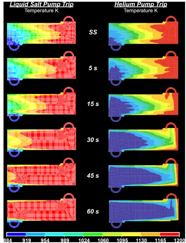
Fig. 5 Transient temperature distributions solved by CHEETAH for the composite plate of the PCHE after a step change in flow rate initiates a thermal hydraulic transient
