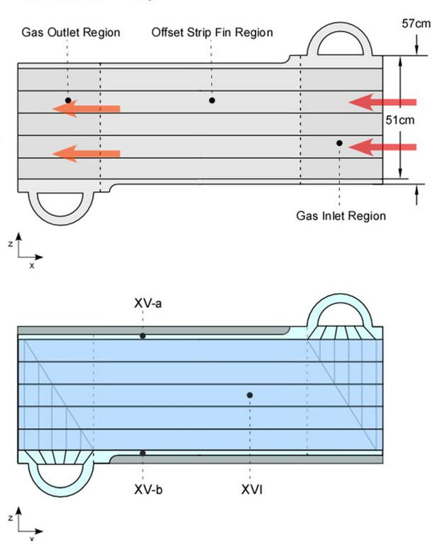
**Fig. 3** Zones in the composite plate with varying thermal and hydraulic properties
