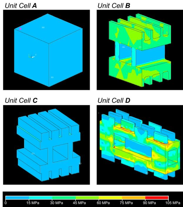
Fig. 8 Local peak stresses on unit cells in the PCHX during a simulated thermal transient involving loss of forced gas heating
