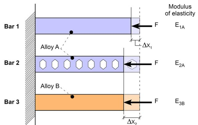
Fig. 6 The strain of a mechanical component with a complex geometry can be replicated with a component with a simple geometry when the two share effective mechanical properties such as an effective modulus of elasticity
